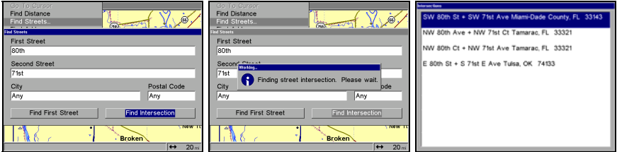
Find Intersection command highlighted (left) and Working message (center). The Intersections Found list (right).
